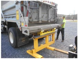
block wall and a sliding mechanism so that a backhoe with forks can lift the spreader off the wall and onto a truck for installation. The system allows the
