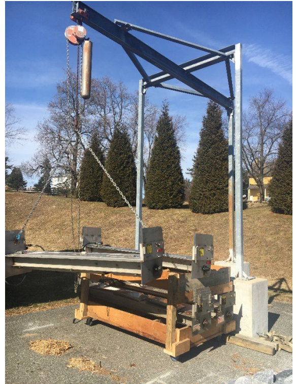
The East Brandywine Township road crew designed a portable storage rack for spreaders using scrap lumber and inexpensive wheels. A hoist lifts the spreaders for mounting on trucks. (Credit: Matthew VanLew, East Brandywine Township, PA)
