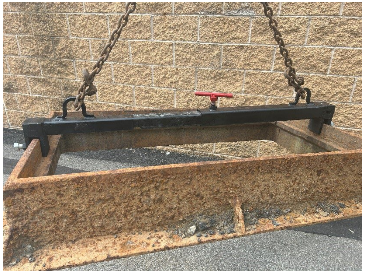
The township designed a tool to safely and conveniently lift storm basins for maintenance. Photo: Peters Township, Washington County
