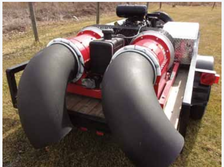
This road ditch cleaner can blow a ditch clean of leaves and debris without removing the beneficial vegetation that holds soil in place. Armstrong Conservation District, 2016 Runner-up
