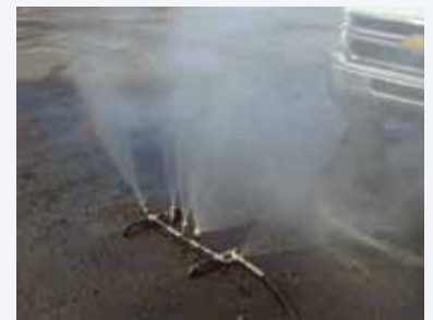
This high-pressure undercarriage sprayer removes corrosive salt and residue from the underside of trucks and equipment. Swatara Township, Dauphin County, 2016 First Place Winner
