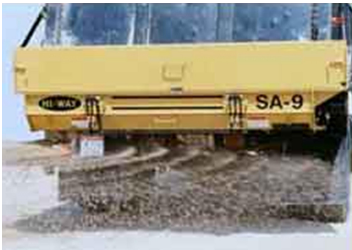
How fast the spreader truck is going will affect the application rate of the salt.
