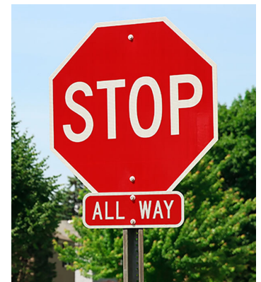
Drivers expect stop signs to be octagonal with a red background and white "STOP" letters.
