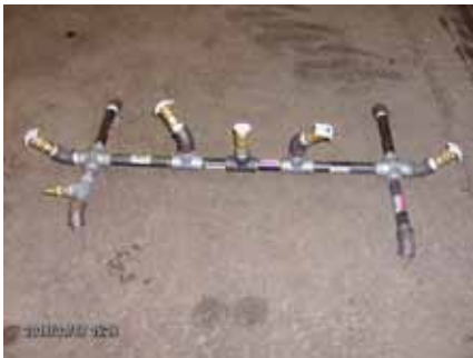
Swatara Township's winning invention: a high-pressure undercarriage sprayer
