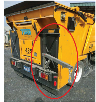
2018 Runner-up: Storm sewer grate hoist, Bath Borough, Northampton County
