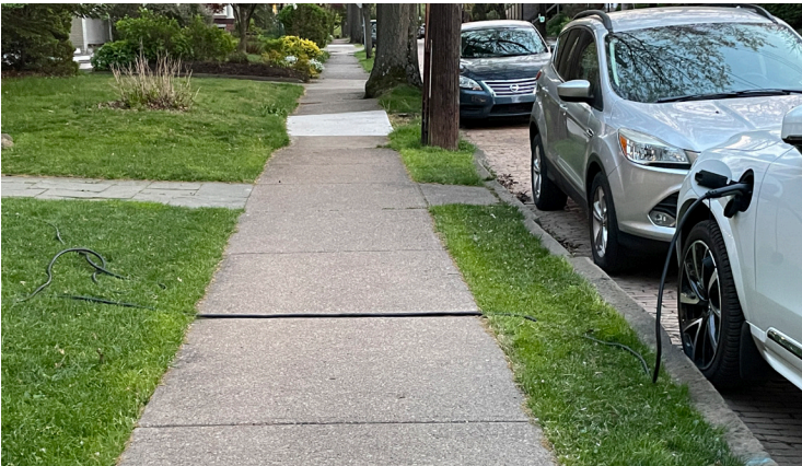
An electric vehicle charging cord lays across a residential sidewalk without a cover. The cord must be covered to comply with federal accessibility regulations and to ensure sidewalk safety for all users. Photo: PennDOT
