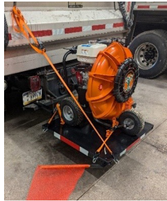
The leaf blower mounted on the back of the truck. Photos: North Centre Township, Columbia County.
