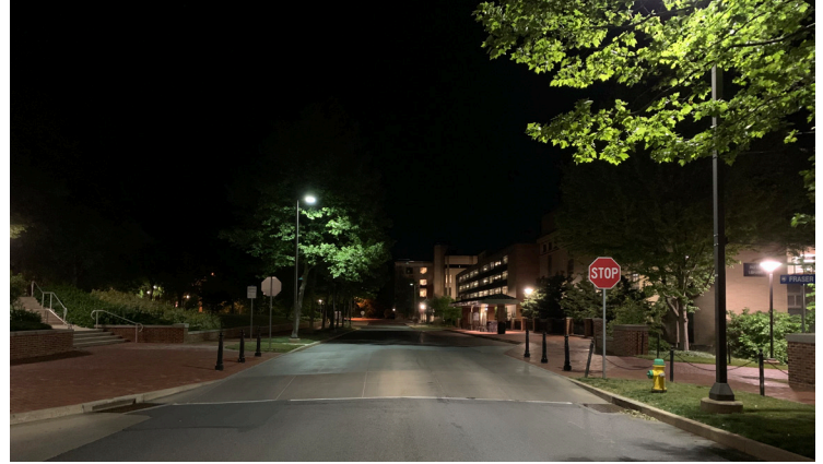
Lighting was used at the crosswalk to improve visibility for drivers to see pedestrians. Photo: PennDOT LTAP
