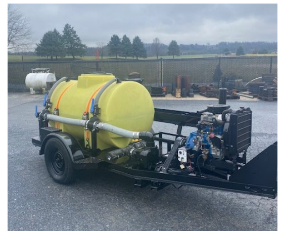
Warwick Township crafted a hydroseeder which made restoration and seeding after projects much easier. Photo: Warwick Township, Lancaster County
