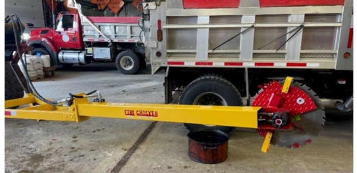
The blade used on the "fire chicken" spins at about 400-500 rpm. Photo: North Codorus Township, York County
