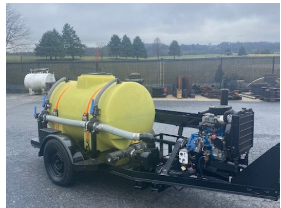
Warwick Township crafted a hydroseeder which made restoration and seeding after projects much easier. Photo: Warwick Township, Lancaster County
