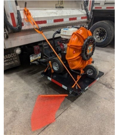
The blower mounted on the back of a truck. Photo: North Centre Township, Columbia County
