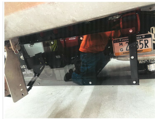
The salt deflector (a metal frame with clear plastic) mounted behind the salt spreader and in front of the back-up camera. Photo: Everett
