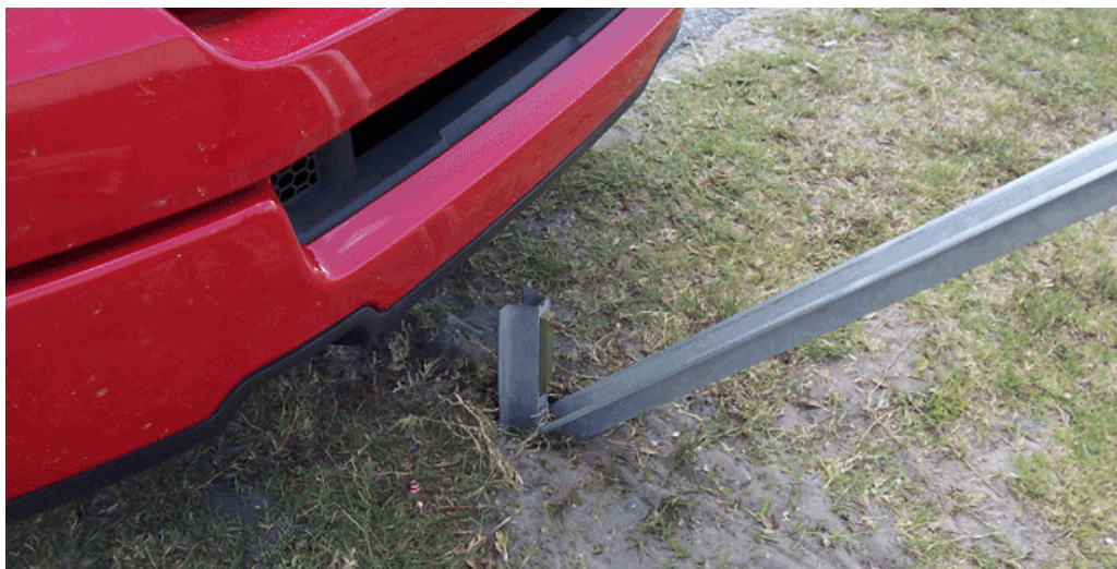
A breakaway post is a crash-tested sign support that, by design, will break or bend upon impact.
