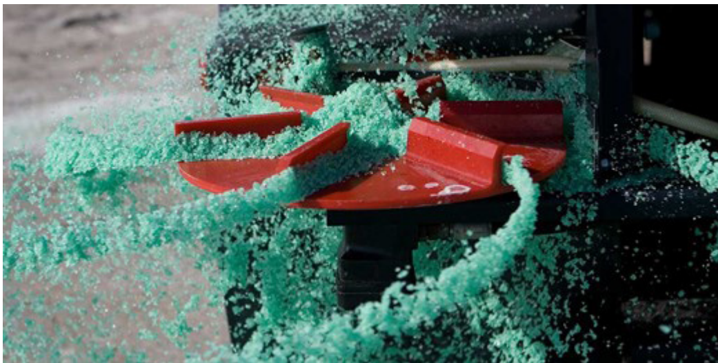
An example of an enhanced chloride deicer with a corrosion inhibitor and coloring agent.
