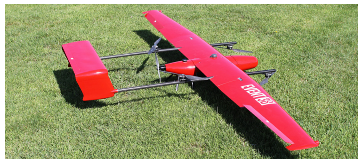
A fixed-wing hybrid VTOL drone can fly long distances. Photo: PennDOT
