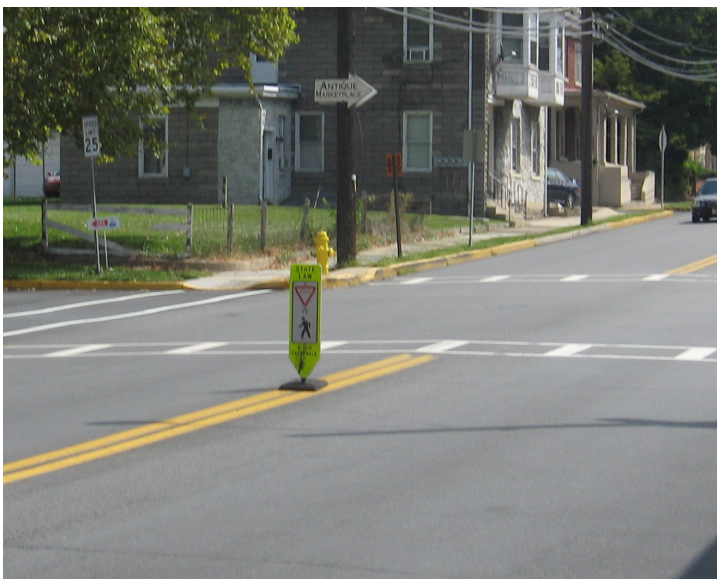
This warning sign along Third Street in Lemoyne Borough, Cumberland County, alerts motorists to a pedestrian crossing.
