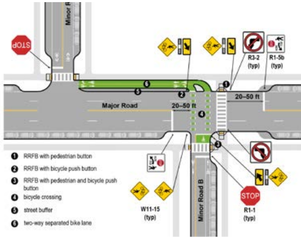
Figure 8-15: Example of Connecting Offset Bicycle Boulevard Segments Using a Two-Way Separated Bike Lane
