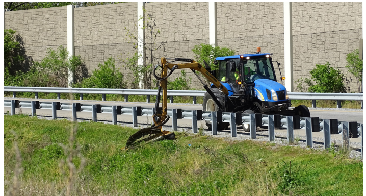
Working from the outside of infiltration/filtration surfaces prevents compaction to the surface. Equipment like this boom arm mower can be used in this fashion.
