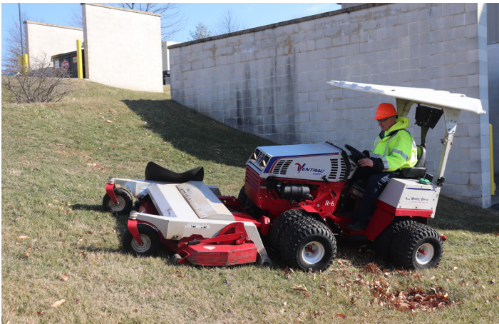
LGP Equipment may use double- or -triple-axle wheel arrangements to carry the equipment load safely using low pressure tires like this Ventrac.
