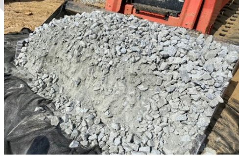
Stone in GSI systems should be clean-washed and not contain fine particles. If washed stone arrives at a construction site dirty, it should be rejected or washed on site. Photo: Cedarville Engineering Group
