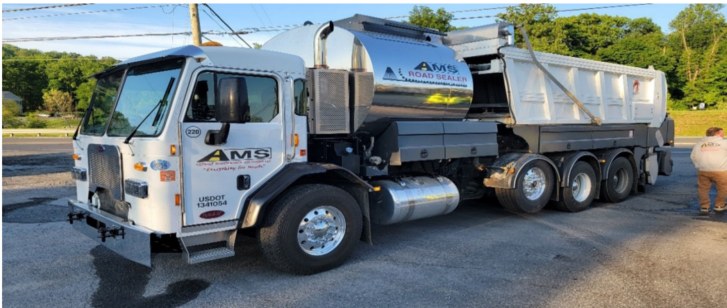
The Self-Contained Skin Patching Truck is a single, truck-mounted unit that does the work of five tandem-axle dump trucks, a chipper, spreader and two oil distributors. Photo: PennDOT
