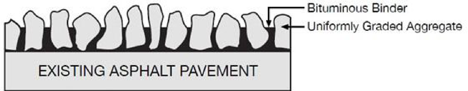
Cross-section of a one-size seal coat aggregate
