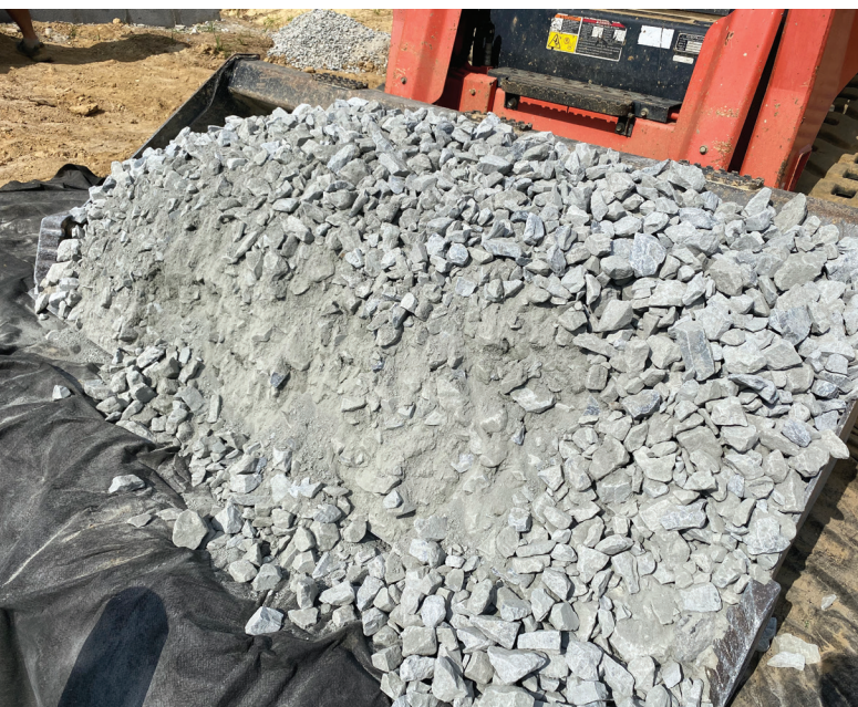
Stone in GSI systems should be clean-washed and not contain fine particles. Even some washed stone can arrive at a construction site dirty, at which time it should be rejected or washed on site. Photo: Cedarville Engineering Group.
