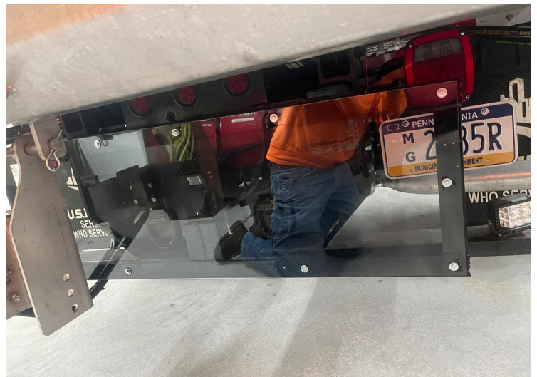
The barrier keeps the salt from going under the truck and the back up camera still works. Photo: Everett Borough
