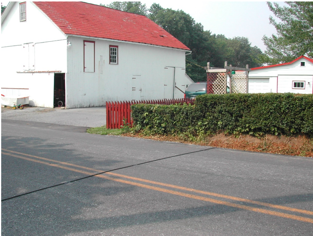
Short-Term classification count installed.
