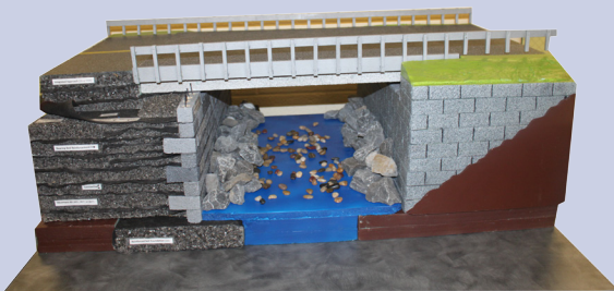
This tabletop model showcases GRS-IBS bridge technology, which is one of STIC's most successful initiatives to date.
