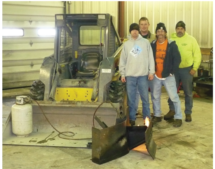
Workers in Richland Township, Allegheny County, show off their winning entry in the 2011 competition. For a cost of $350 in materials and labor, they built a curbing attachment for their skid steer so that they could create nicely shaped and straight curbs.
