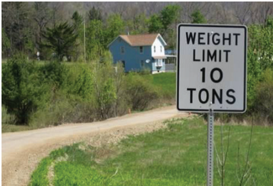
Posting weight limits on a secondary road is the first step in ensuring that a municipality's roads are protected from heavy haulers.
