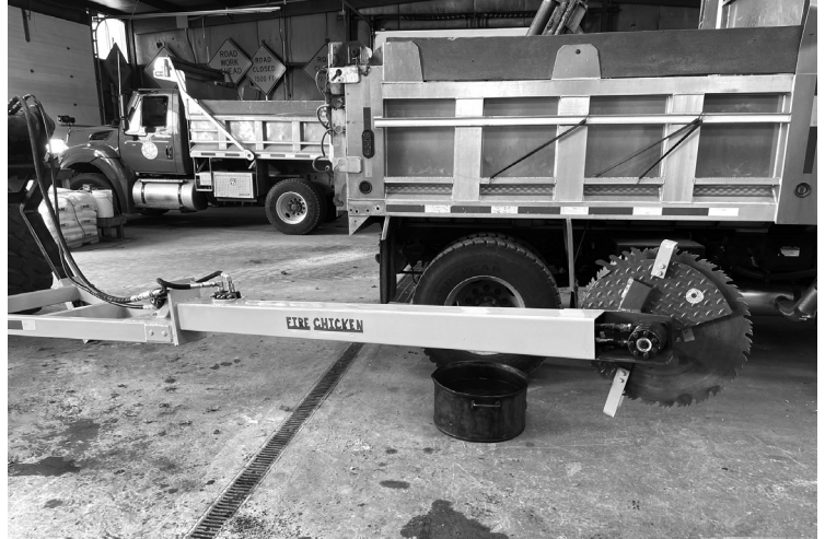
The blade used on the “fire chicken” spins at about 400-500 rpm. Photo: North Codorus Township, York County
