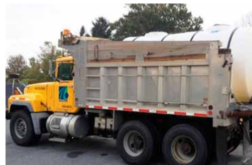
Tandem-axle dump truck retrofitted with 1,000-gallon insert
