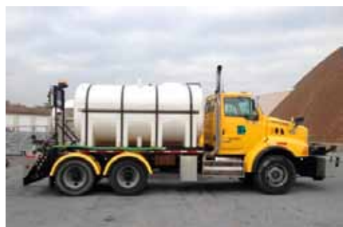
3,000-gallon anti-icing tank
